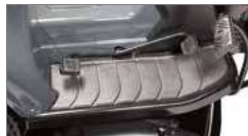
New side-discharge lawn tractors with speed controlled by means of a double pedal that acts directly on the hydrostatic transmission. This solution allows reversal of the direction of travel and precise speed control during operation.
