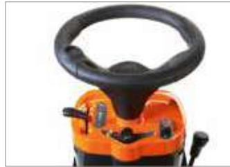
The electromagnet clutch is engaged quickly and quietly by way of a handy dash-mounted button.
