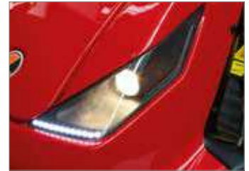
Halogen headlights and LED worklights ensure a good view of the cutting area, even in low light conditions.
