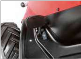
Self-locking differential for the maximum traction in all conditions of terrain and gradient.
