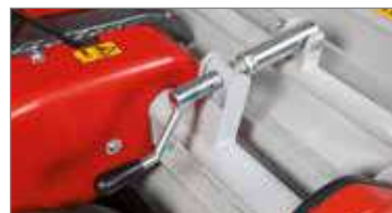
Easy cutting height adjustment by means of a worm screw lever.
