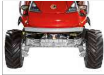
The large tyre footprint and low centre of gravity combine to maximise stability of the machine, even on steeper gradients and when working alongside verges and ditches.
